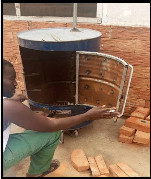
Fig. 14: Complete skeletal structure of the oven Fig. 15: Sizing of the brick by cutting
